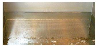
Add oil until the oil level is at the top OIL LEVEL line. DO NOT OVERFILL THE FRYPOT.
